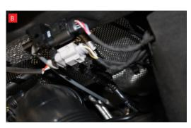
A) Remove Lambda Probe from OE catalyst, then remove cable from clips indicated. (x4)
